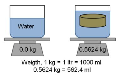
**Figure 7.** Water replacement method with weight. Note; scale must be set to zero before putting the sample disk into the water.
