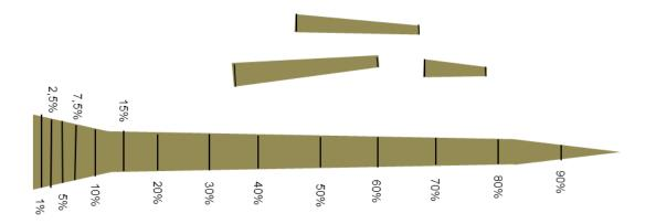
**Figure 6.** The 14 relative heights marked on the stem showing the points where the over- and under-bark diameters are measured for volume estimation. In addition, the sample branch sections with a diameter  $\ge 2$  cm are measured for volume estimation.
