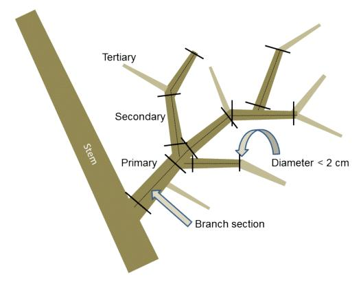
**Figure 4.** Measurement of sample branches for volume by sections. The branch sections with top diameter less than 2 cm are weighed for biomass, separately for branch wood and foliage. However, for t thorny species they are weighed together.
