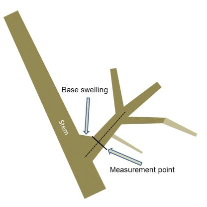
Figure 5. Measurement point of branch diameter in case of base swelling or other deformity.
